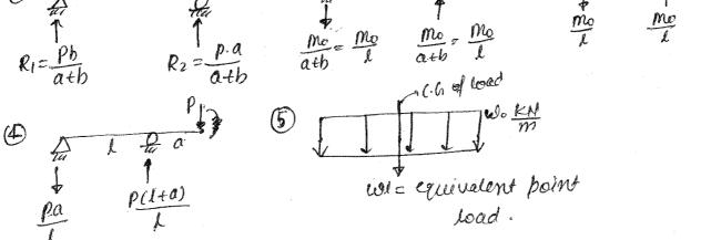
Distributed loading like UDL, UVL etc can be toleated as a point load having magnitude equal to area of the load distributed diagram & passing through the C-G of load distributed diagram (only for reactions calculation).
